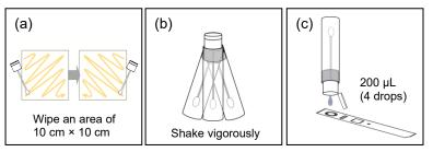
Fig. 2. Test steps for swab test sample
